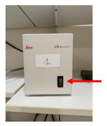
2- Turn on the joystick. The switch is on the back.
